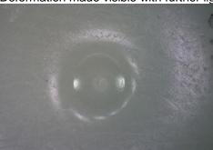
The indent diameter result is based on material properties only, not surface structure. Several tests have resulted in the observation that in nearly all cases the surface of the indent is smooth and reflects light (see 5.4). If the surface of glare material is made rough before the test by sanding, the edge to be observed appears more distinct.
