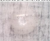
It must be noted that any procedure making the indent visible after the ball pressure test must be possible to make within 3 minutes including the measurement itself (see cl. 8.4 b).
